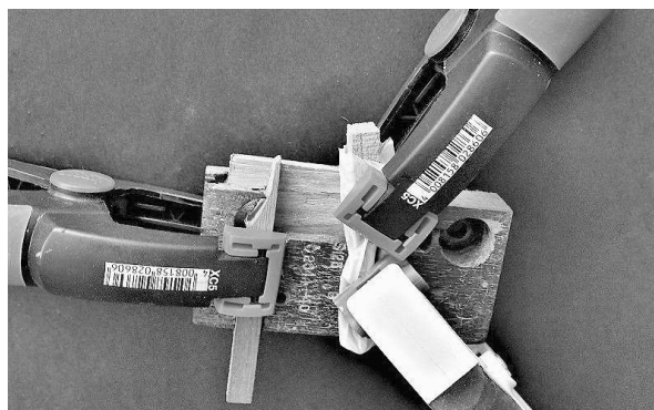
John's repairs to the damaged key base in progress.
