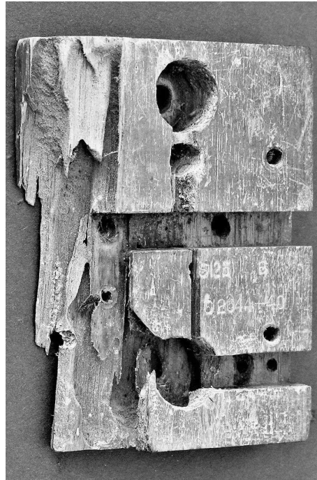
A closer look at the borer (Lyctus Beetle) damage underneath the base of the PMG key.
